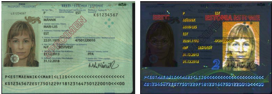
Figure 4–9: Passport (EST, P, 1, 2013): Verify the facial image in the visible light image against the one printed with UV-luminescent ink
