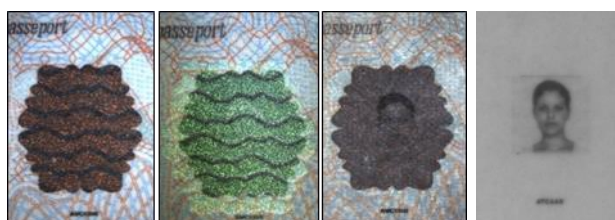
Figure 4–3: Passport (HUN, P, 1, 2006): Personalized OVI viewed under two different angles, under transmitted light and under IR light
