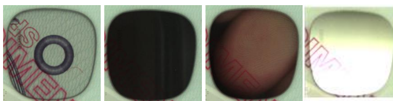
Figure 4–7: Passport (SWE, P, 1, 2012): Window feature with variable content; from left to right: inner front cover; reader housing; fingertip; glare induced by incident light
