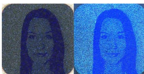
Figure 4–4: Passport (LVA, P, 1, 2015): “Negative” personalization through laser engraving under different viewing angles in visible light
