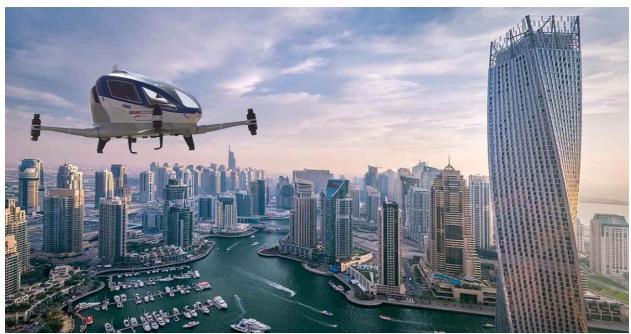
The Ehang184 prototype from China is one of a number of new remotely piloted aircraft being designed to function as aerial taxis, or for related operations at low altitudes. It features pre-set routes which passengers select from upon entry. If current plans in the UAE remain on track, it could begin carrying travellers from the city's main airport to downtown Dubai as early as July of this year.
