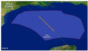
SBS program will provide ATC with surveillance for non-radar regions in the Gulf of Mexico allowing radar-like separation (~ 5 miles in trail), as opposed to current non-radar procedural separation (~ 50 miles in trail)
