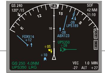
FIS-B transmits graphical National Weather Service products, temporary flight restrictions (TFRs), and special use airspace to ADS-B In
