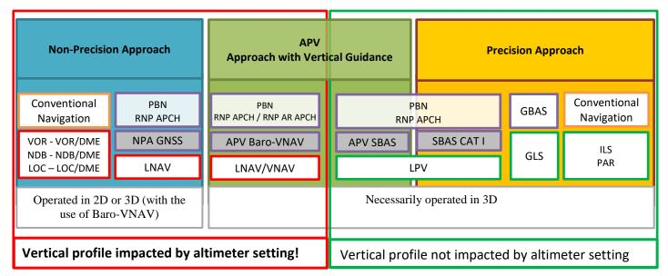
Figure 2 – Approach procedures and Altimeter setting
