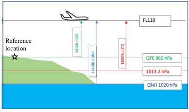
Figure 1 – Altimeter setting
