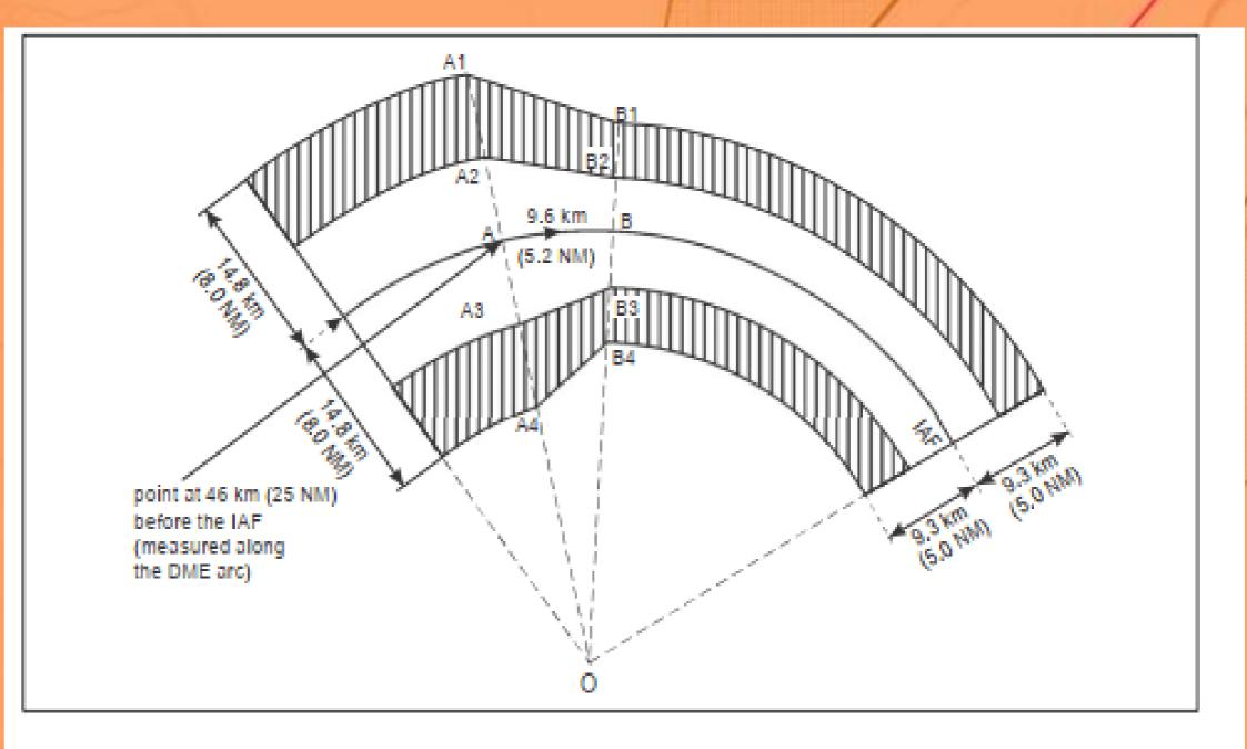
Figure I-4-2-3. DME arc — length of the arrival segment greater than or equal to 46 km (25 NM)
