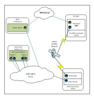
Figure 1: Curacao SDP Network Architecture
