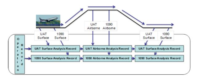
Illustration of how data is collected in operation and analysis records
