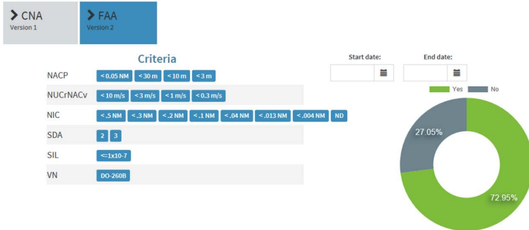
Fig. No. 7.- Example of ADS-B Performance level establishment to filter data
