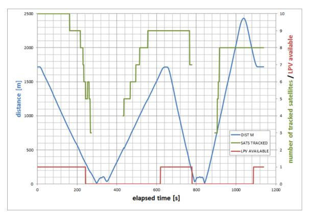
Effect of moving Jammer 4 on Ashtech aircraft GPS receiver – the longest loss of the LPV
