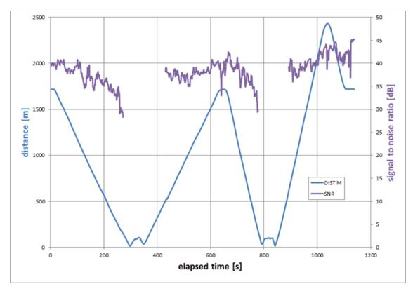
Effect of moving Jammer 4 on Ashtech aircraft GPS receiver's S/N ratio
