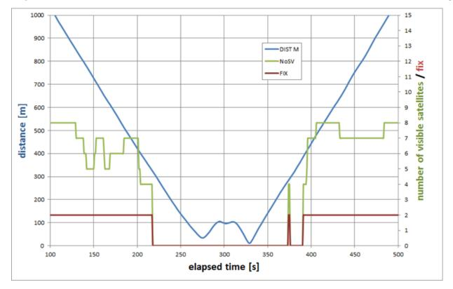
Effect of moving Jammer 2 on Hemisphere DGPS receiver
