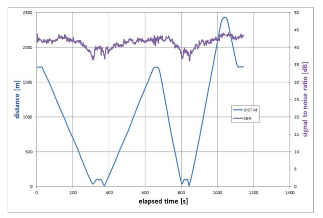
Effect of moving Jammer 3 on Ashtech aircraft GPS receiver's S/N ratio
