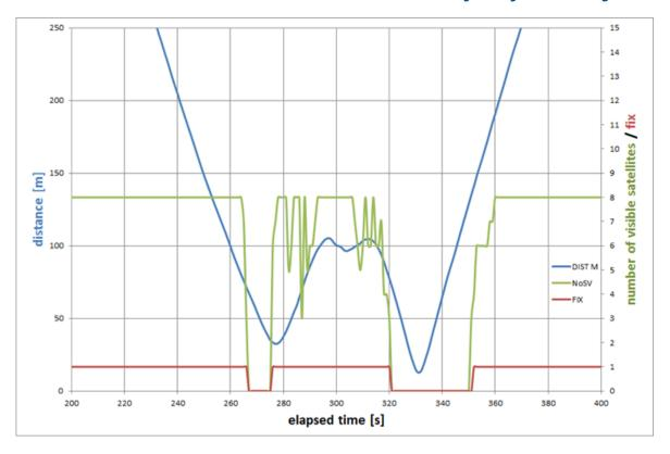
Effect of moving Jammer 2 on Squid/ERA receiver
