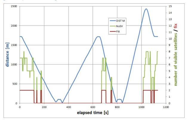
Effect of moving Jammer 4 on Hemisphere DGPS receiver
