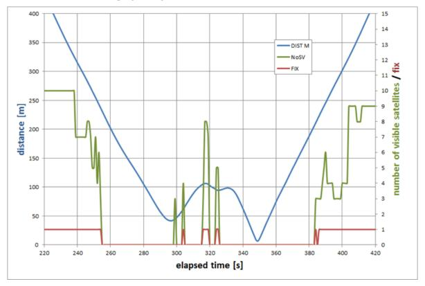
Effect of moving Jammer 4 on Squid/ERA receiver
