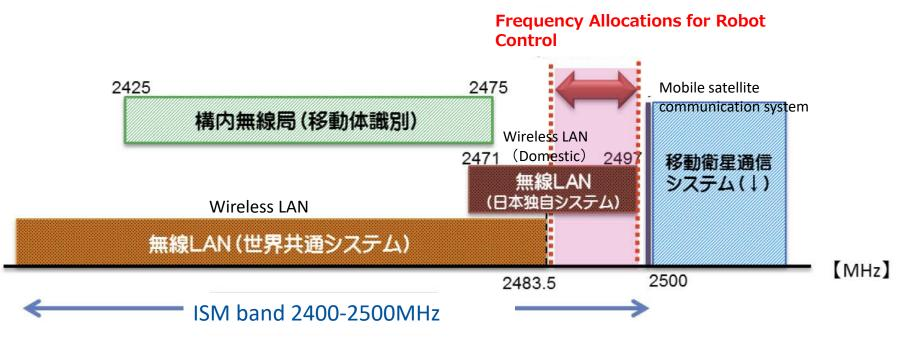
Figure Frequency allocation of 2.4GHz band
