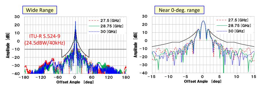
Measured off-axis radiation patterns
