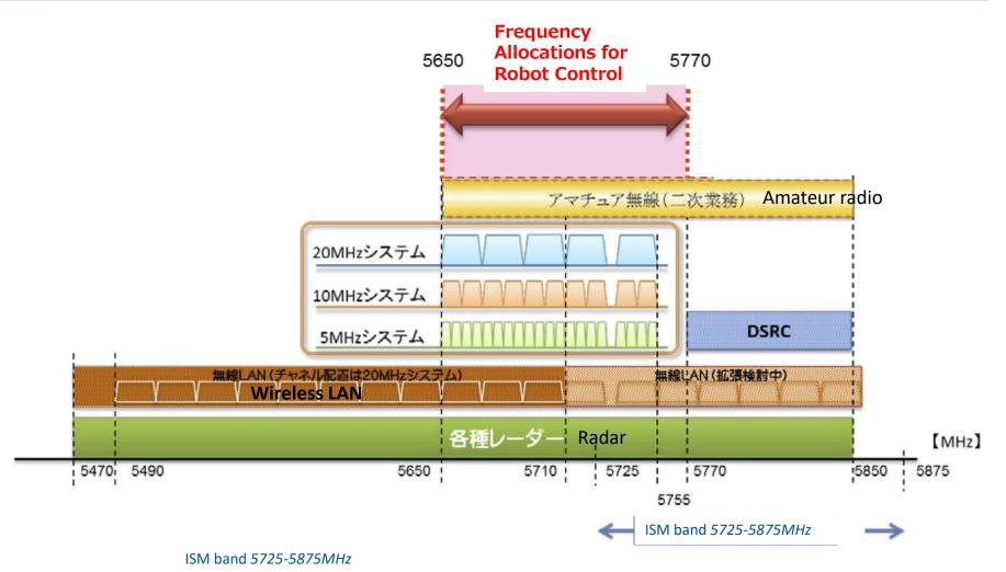
Figure Frequency allocation of 5.7GHz band
