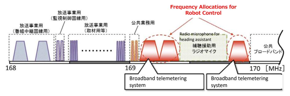
Figure Frequency allocation of 169MHz band
