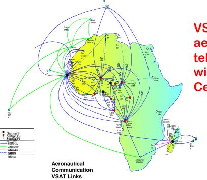
VSAT networks for aeronautical ground-ground telecommunications are in wide use in both Africa and Central/South America
