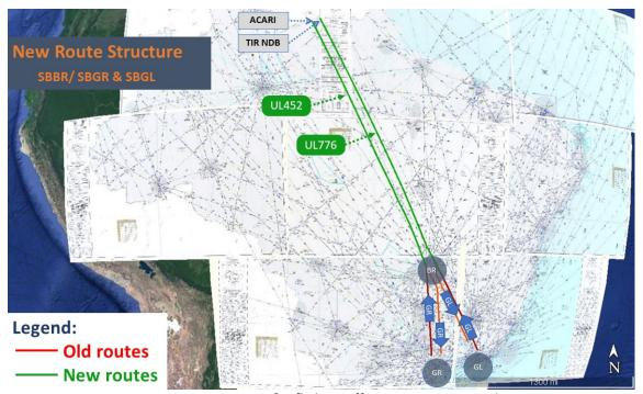
Figure 2 – New structure for flights to/from SBBR, SBGR and SBGL
