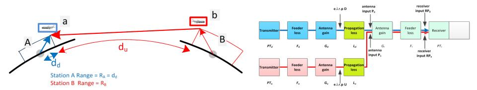
Minimum separation between stations A and B: Range A + Radio horizon A + Radio Horizon B + Range B
