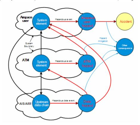
Figure 4: AIS/AIM data hazard model (CHAIN Safety Plan)
