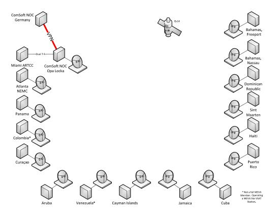
2.4 The Network is capable of fully-meshed voice communication. Any node can call any other node provided such call is allowed by the MEVA Dialling Plan. Beside voice lines a number of shout lines are implemented allowing Air Traffic Controllers to immediately talk to their counterparts without dialling.
