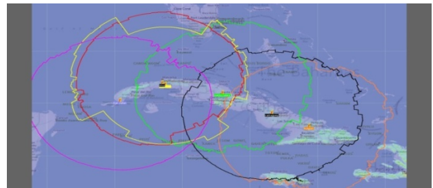
Fig. 1 ADS-B Coverage at 33000 feet in Habana FIR
