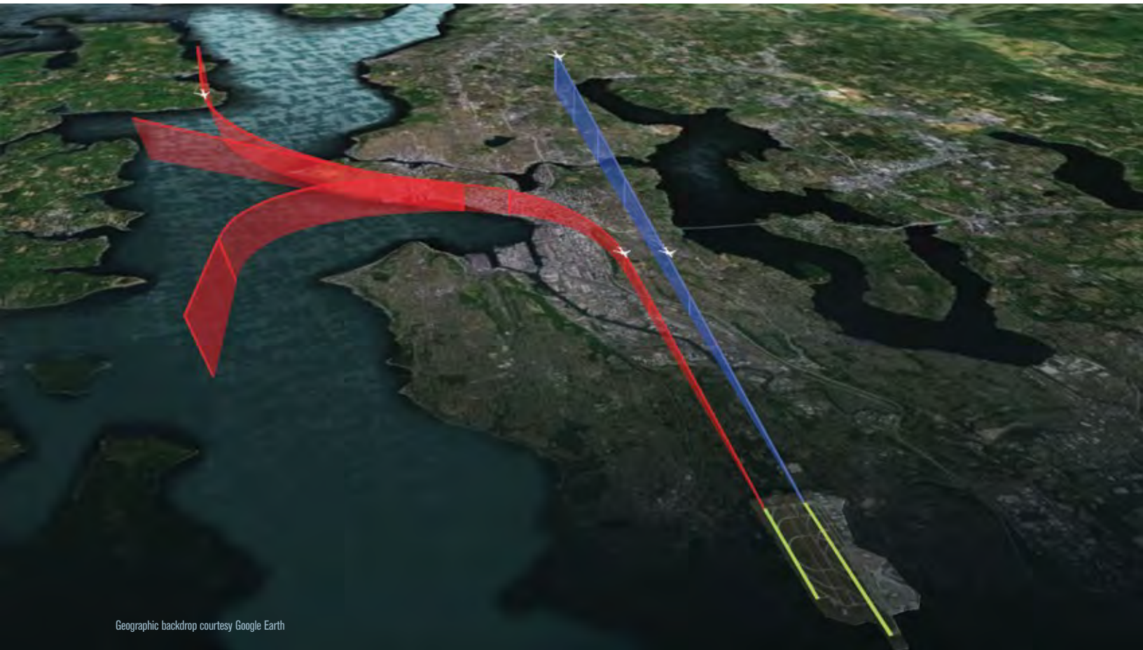
Fig. 7: PBN as an enabler for optimization of closely spaced parallel runway operations.
