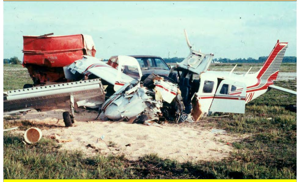
This incident occurred when a pilot lost control of the aircraft during takeoff and hit a grain trailer parked in the runway strip.
