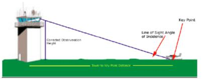
Figure 4 Representation of Tower to Key Point Distance
