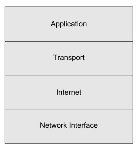
Figure 1-2: TCP/IP Layer Model
