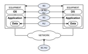
Figure 5-2: Technical Controls to ATN Component Mapping
