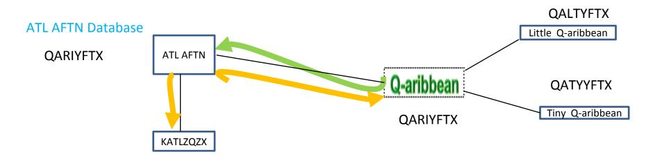
A user in Q-aribbean, sends an AFTN message to the ATL AFTN center, addressed to KATLZQZX (an Area Control Center) and QARIYFYX (an AFTN office on the Main island).
