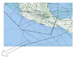
Lack - deficient AMS VHF Communications in routes close to the Pacific coasts – near Acapulco and boundary with Central America FIR
