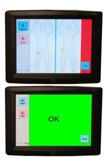
Operators are presented with an "objects detected screen" signifying specific location(s) on the passenger when anomalies ARE detected.
