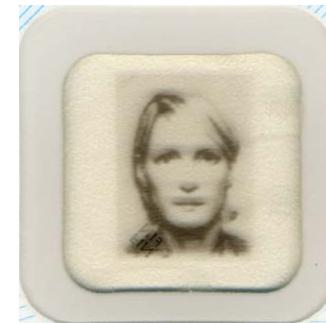
Reverse side in transmission: Mirrored image visible from other side.
