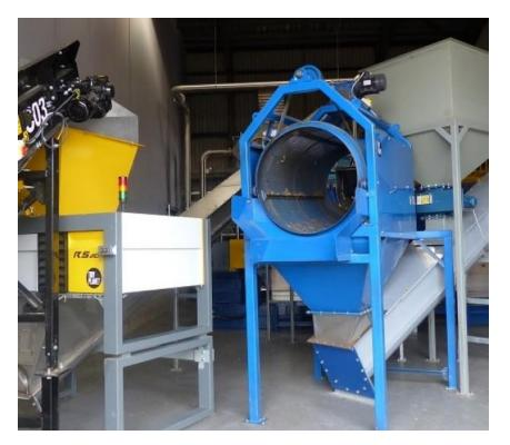
• Waste is prepared by shredding, screening, and drying.
