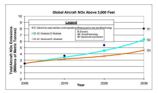
Figure 3. Total Global Aircraft NOx Above 3,000 Feet AGL.
