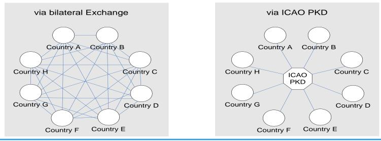
This example shows 8 States/non-States requiring 56 bilateral exchanges (left) or 2 exchanges with the PKD (right) to be up to date with DSCs and CRLs. In case of 192 ICAO States 36,672 bilateral exchanges would be necessary while there are still 2 exchanges with the PKD.
