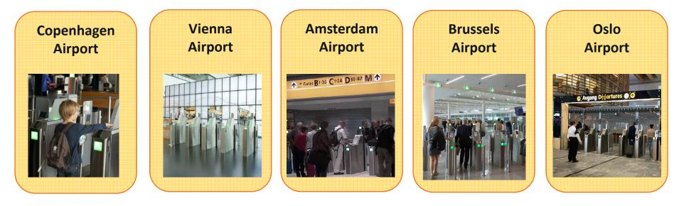
Scan boarding pass, verify flight data and open gates
