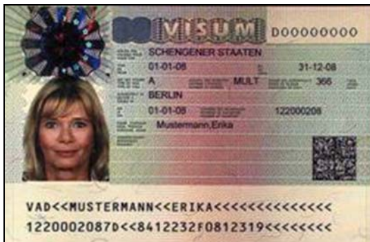
Example of a MRV showing the digital seal For enhanced security, the IR-readable barcode could partially cover the portrait (Source: BSI)
