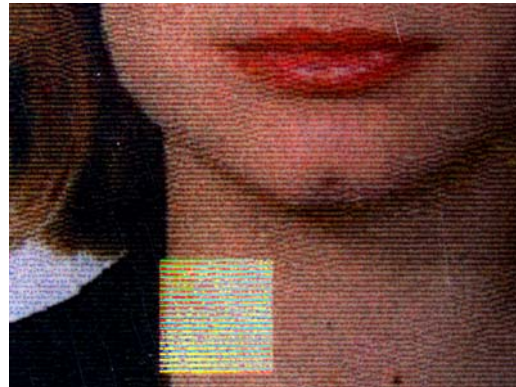
Machine verifiable DOVID structure within the transparent overlay of a Bulgarian passport (square region in the image above)
