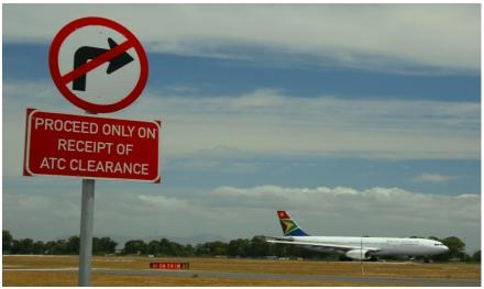
Clearly signed vehicle roadway entrances that lead to taxiways and which give clear instructions to seek ATC clearance before the vehicle can proceed onto the taxiway
