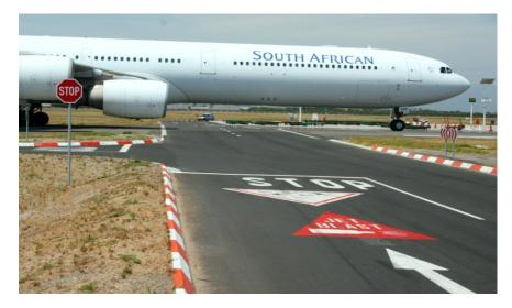
Clearly marked and signed uncontrolled vehicle crossing points, as per ACI recommendations, now at all locations on all service roads and perimeter tracks
