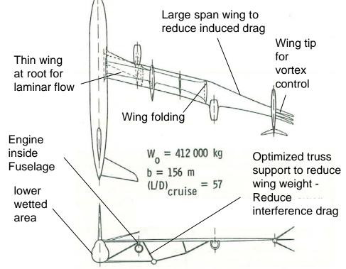
• Revolutionary: If successful, this design will Double the Lift/Drag ratio of a conventional transport aircraft
