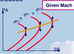
When ATC allows them, step climbs are performed to stay close to the optimum.
