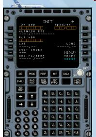
Indeed, flying at a given Cost Index provides the benefit of flying at the Optimum Mach Number as a function of aircraft weight, flight level and wind component.
