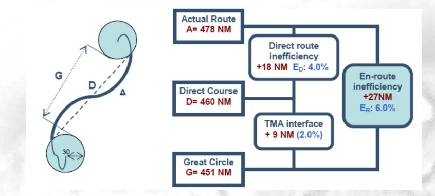
Distance shown are average for all city pair in Europe in 2005. Where the flight originates or ends outside Europe only the portion of flight inside the IFPS zone has been taken into account
