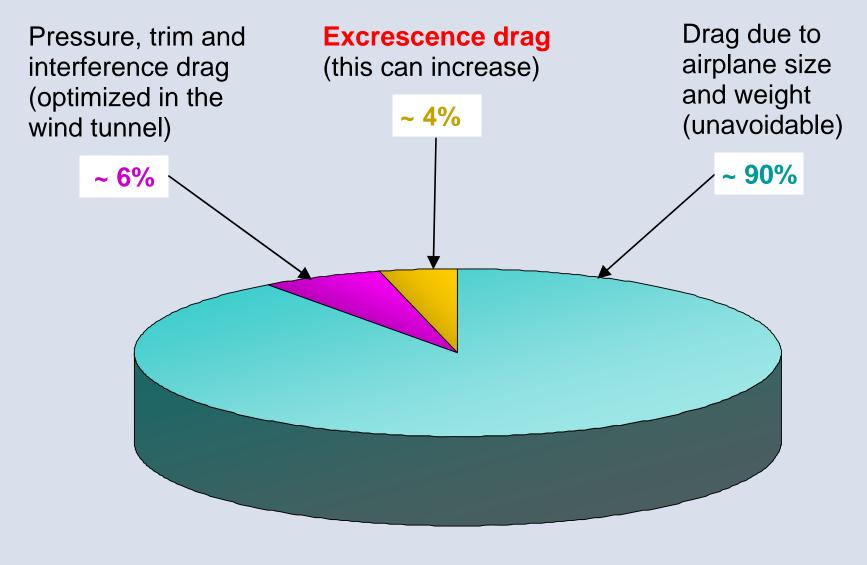
The additional drag on the airplane due to the sum of all deviations from a smooth sealed external surface
