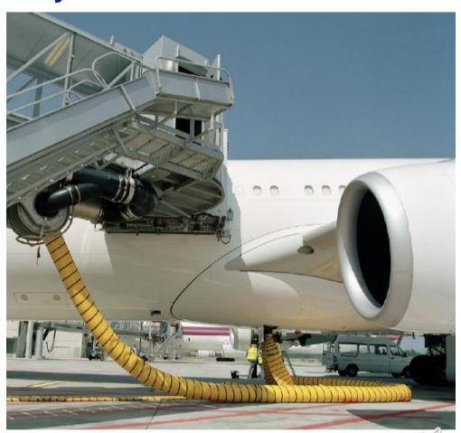
Ducting for Pre-Conditioned Air (PCA)
