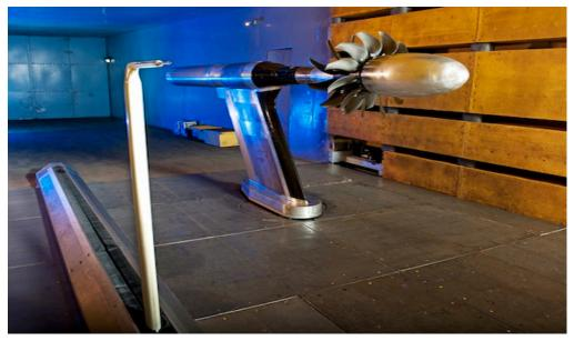
Open Rotor Propulsion Rig installed in GRC's 8x6 and 9x15 Wind Tunnels (GE)
