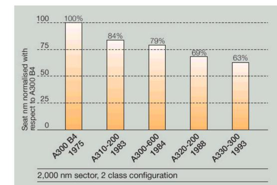
Comparative fuel consumption of Airbus twinjets Source: The Airbus Way -Environment July 2002
