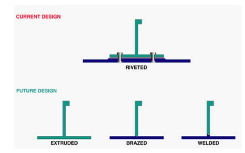
welding: Fuselage structures using integrally stiffened panels, extruded or with welded-on stringers, compare very positively in terms of weight and durability with today's riveted structures where additional thickness has to compensate for the rivet holes.
