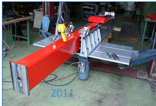
Installation at SR Technics, including retractable sampling probe
