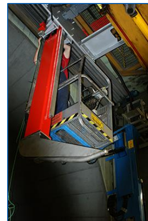
Installation at SR Technics, including retractable sampling probe
