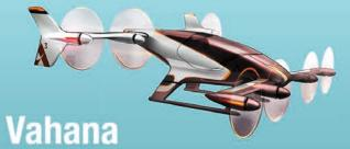
A single-passenger, self-piloted electric vertical take-off and landing (VTOL) aircraft being developed to open up urban airways.
