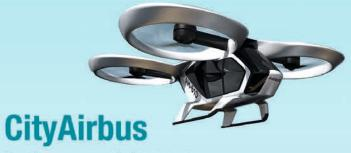
A multi-passenger, self-piloted electric vertical take-off and landing (VTOL) demonstrator designed for urban air mobility with cost efficiency, high-volume production and a low environmental footprint in mind.
