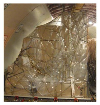
Typical cargo pallet built to best contour - 96/96/125" side by side (A330-200F shown)
