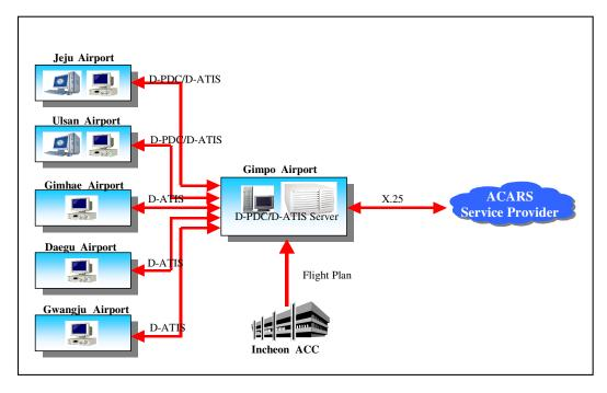
Figure-2. Configuration of the D-PDC/D-ATIS systems
