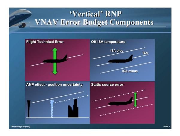
Figure 3 - 'Vertical' RNP - VNAV Error Budget Components
