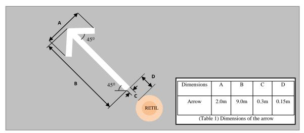
Figure 2. Dimensions of the rapid exit taxiway indicator markings
