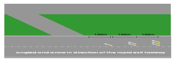
Figure 1. Example of rapid exit taxiway indicator markings
