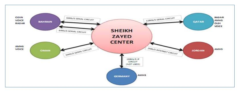
Figure 5: Abu Dhabi Circuit Diagram
