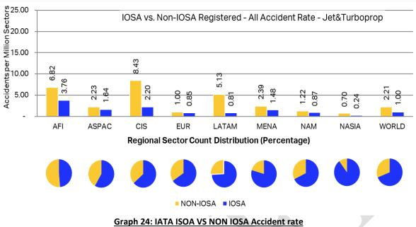
The full year accident rate for IOSA carriers in 2019 was lower than the rate for non-IOSA operators.
