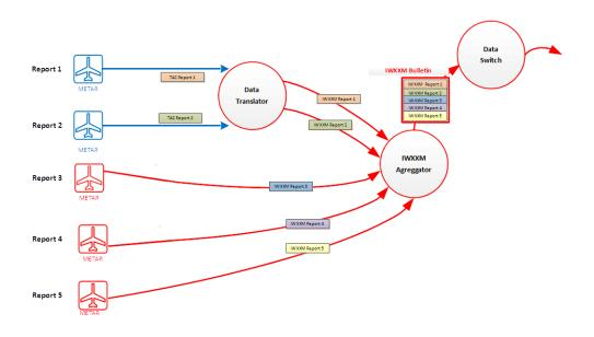
Figure 4: Aggregation of TAC and IWXXM data
