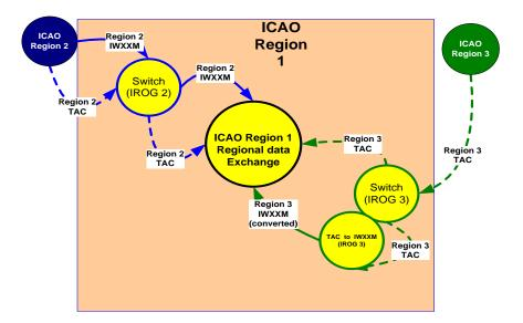
Figure 6: Phase 2, interregional exchange of OPMET with Region 2 (IWXXM & TAC capable) and Region 3 (TAC capable)
