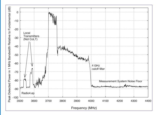
Measured emission spectrum of a typical 5G base station (NTIA Report)
