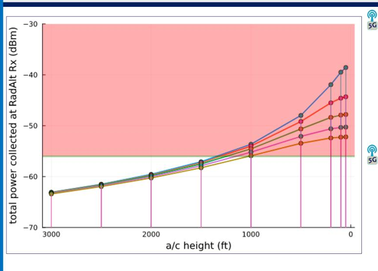
The calculations of the total OOB interference power from the 5G intentional emissions in the allocated frequency band reaching the front end of the RadAlt receiver. The Figure shows plots of the power at the RadAlt receiver expected to be caused by the various base station locations.
