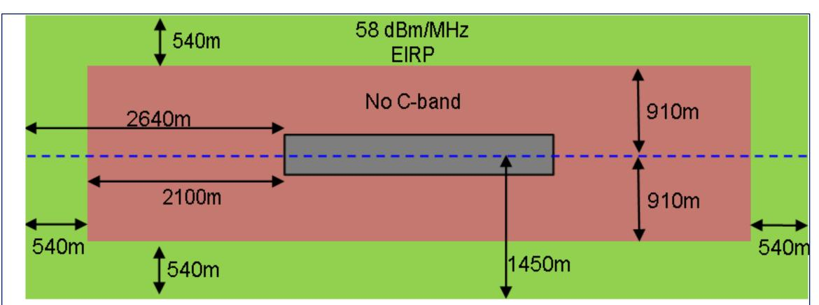
Note: This illustration is for guidance on the protection zones at an aerodrome. The green area is defined as buffer zone that depends on the location of BS and several other factors.
