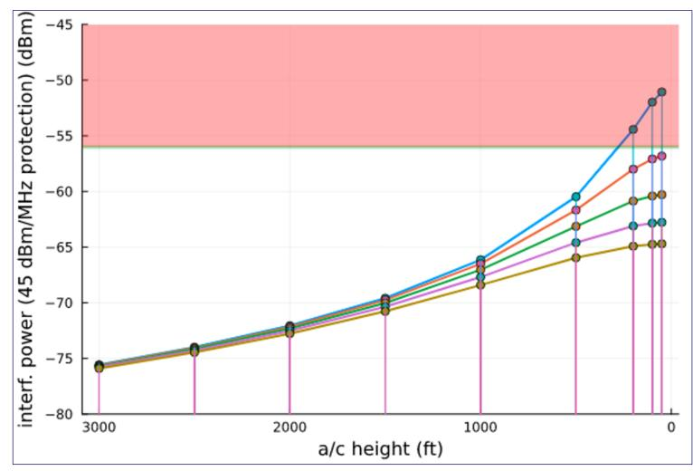
The 45 dBm/MHz protection can greatly reduce the probability of interference power exceeding receiver blocking specification for worst-case RadAlt specification if no 5G base stations are within 2000 meters from runway threshold
