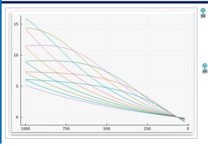
The depression and elevation angles during such approach, angles were computed for nearest and furthest base stations from an aircraft altitude of 1000 ft until touchdown during normal landing procedure
