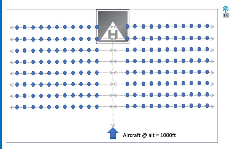
The 5G base station locations considered in the simulation were distributed alongside the approach line to a heliport with constant separations. 20-meter base station antenna heights were assumed
