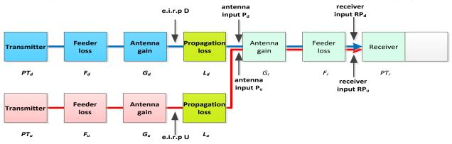
Determine the desired signal level at receiver input
