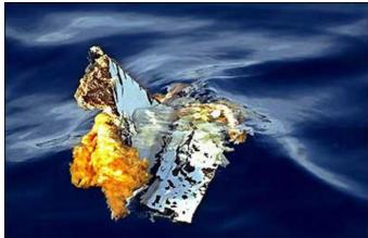
Left turn to intercept VOR after takeoff Aircraft banked right after heading select Co-pilot warned that bank was increasing Captain neutralizes wheel, then increases right bank Banks 111 degs and 43 pitch down Airplane hits water at 24 degs right bank and 4G's
