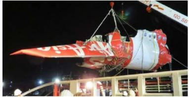
Repeated Rudder Travel Limit Unit failure at FL320 Alternate law entered after reset of FAC CBs Sideslip from rudder causes roll and rise of FD Pilot flying inputs results in stall Continuous stall warning during last 3 mins
