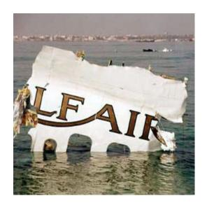
On second go-around, captain command half the pitch req'd and did not maintain runway heading With TOGA and low pitch, aircraft rapid accel Flap overspeed warning; commanded flaps up Captain deflected stick forward and got -15 deg pitch Did not respond to multiple GPWS alerts
