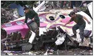
Two go-arounds in low visibility On third attempt, runway not visible at MDA Autopilot disconnected, and captain decides go around Pitch increases to 40 degs, countered back to 32 degs Counter inputs stop and pitch to 48 degs, airspeed 100 Stall
