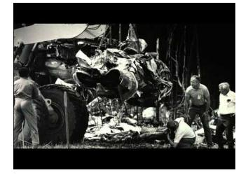
Right engine failure on takeoff at 450 ft Correct then incorrect pedal, followed by aft column
