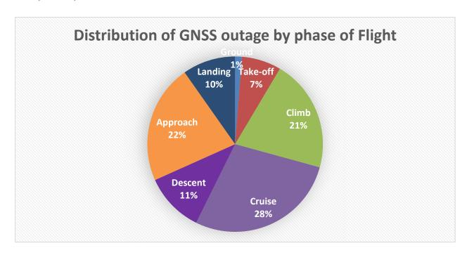
The data shows that the highest GNSS Outage occurred during the phase of flights cruise, approach, climb, and descent.
